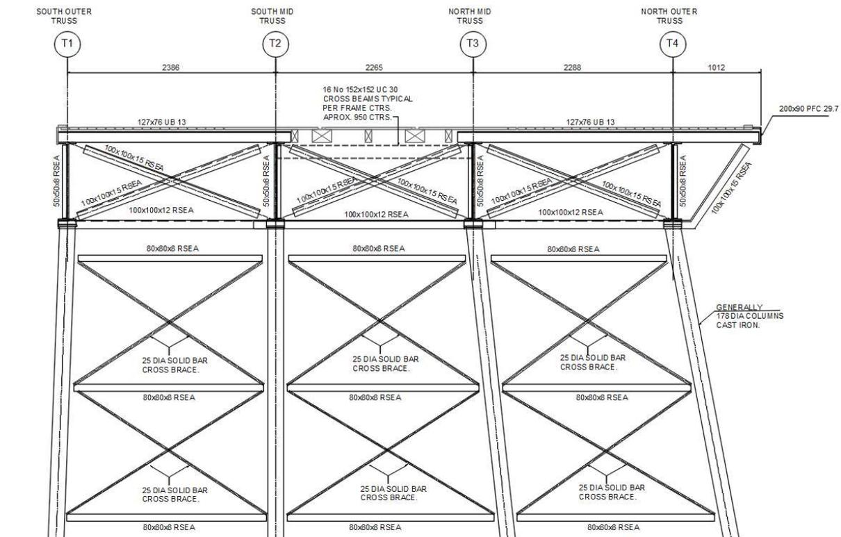
Figure 5 – Typical elevation on beach support frame
