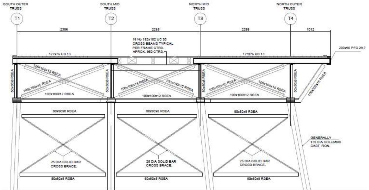
Figure 3 – Typical frame elevation
