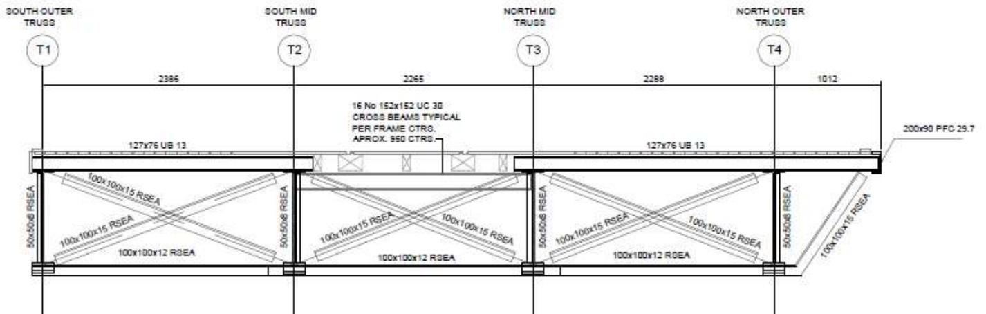
Figure 2 – Typical section through deck
