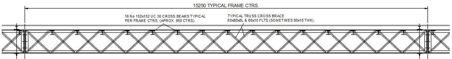
Figure 4 – Typical elevation on longitudinal truss
