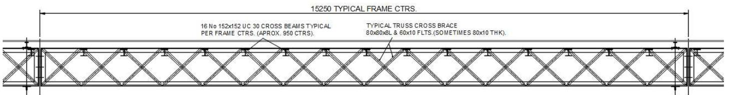
Figure 4 – Typical elevation on longitudinal truss
