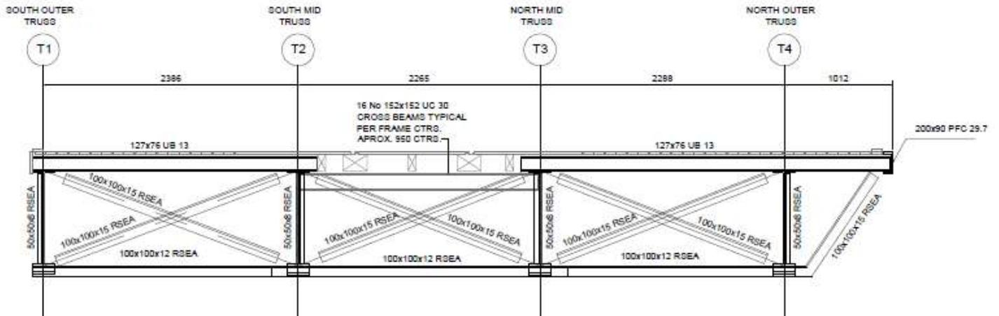
Figure 2 – Typical section through deck
