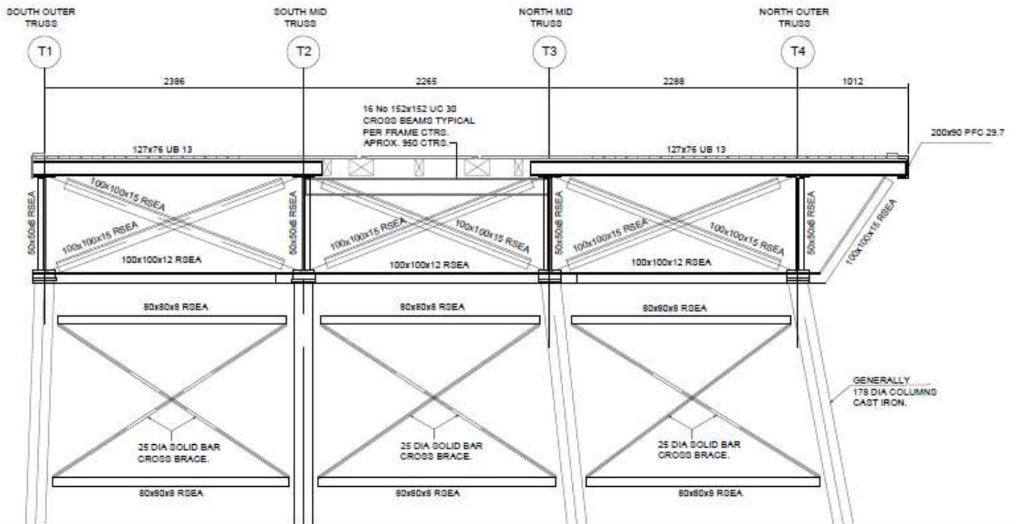
Figure 3 – Typical frame elevation
